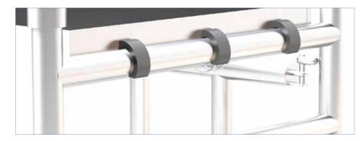
1.11 Place additional frame into base unit and clip in place.
