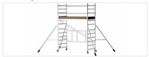
1.17 Add additional frames by climbing through the hatch then place hatch deck at required platform height. Secure hatch platform with locking braces, repeat steps 1.11,1.12, 1.13 & 1.15
