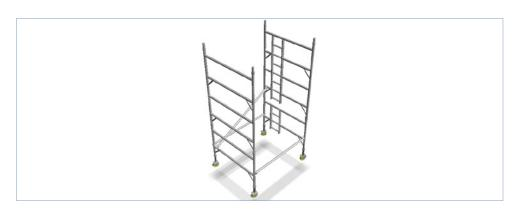
1.11 Clip diagonal braces onto the lowest rungs.
