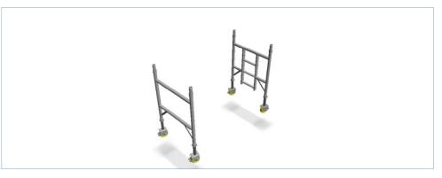
1.5 Clip horizontal brace onto span frame. Connect the brace directly above the casting at the first horizontal rung position. And then attach to ladder frame.
