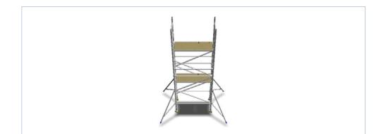
1.36 Climb ladder and open trapdoor. Sit with feet through the platform with both feet on the ladder. Fit four guardrail braces on the 9th & 10th rungs directly above the sides of the platform.
