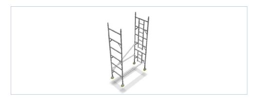
1.11 Clip diagonal braces onto the lowest rungs.
