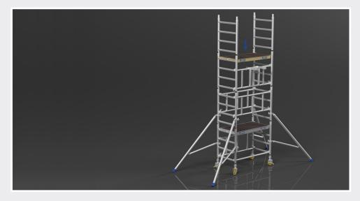
10. Climb internally and from the seated position place the advanced guard rails on the 14th and 16th rungs. – ensure the hooks are locked.
